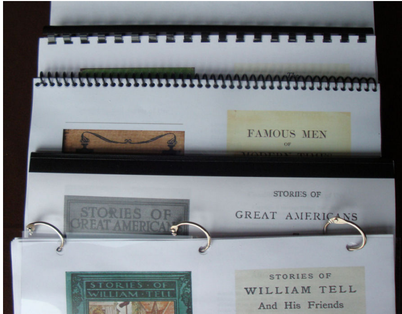
From top to bottom: Comb binding, spiral binding, thermal binding, ring binding
